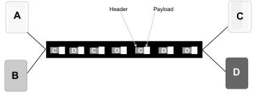
Figure13: Packet Switching Example
