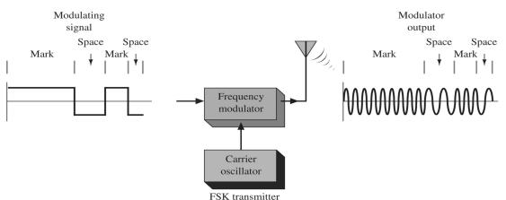
Figure 10: FSK Modulator
