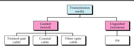
Figure 2: Classification of Transmission Mediums
