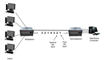
Figure 5: Digital Transmission using TDM
