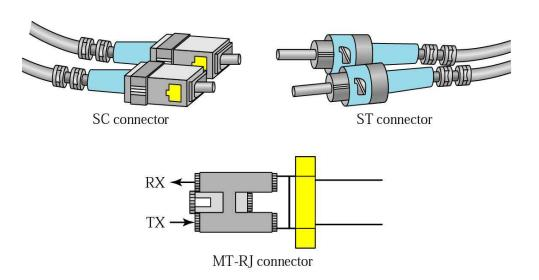
Figure 10: Fiber optic cable connector
