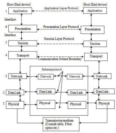
Note: Subnet is the part of the network to which end-devices (Hosts) are attached
