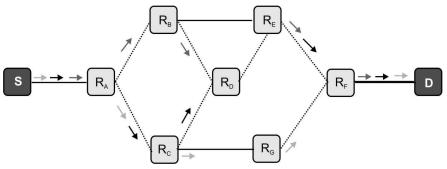
Figure 14: Connection less Packet Switching
