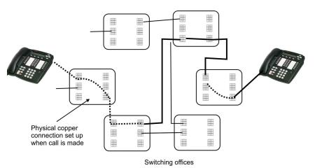
Figure 11: Circuit Switching in the Telephone Network
