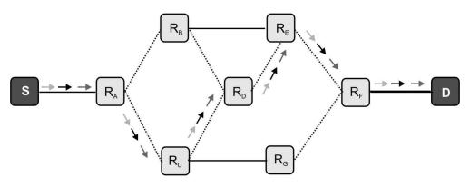
Figure 15: Connection Oriented Packet Switching
