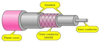
Figure 5: Coaxial cable
