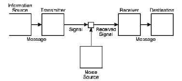
Figure 2: Shannon's diagram of a general communications system
