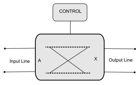
Figure 9: A Simple 2 X 2 Switch
