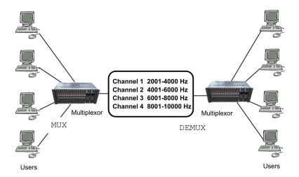
Figure 3: Illustration of FDM using four different channels
