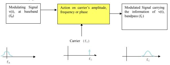
Figure 1: Process of the Analog Modulation
