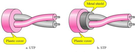
Figure 4: UTP and STP Cables
