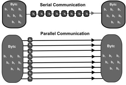
Figure 1: Serial and parallel communication
