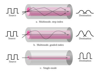
Figure 7: Types of Optical Fiber Cables
